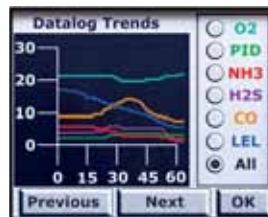
View datalog trends and direct readings graphically.
