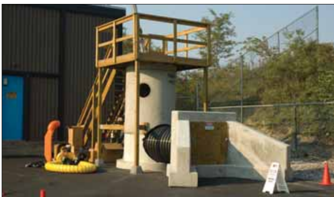
Confined space simulator
